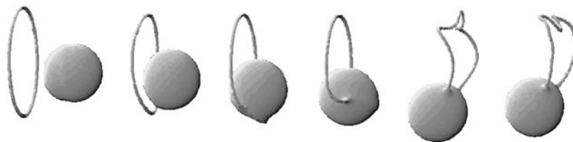
Figure 2. Capture of the stationary ion by the vortex ring: the results of numerical integration of (43), (44) for the isosurface \rho = 0.2 .
